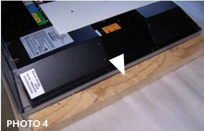
Position the wood stile onto the side of the TV frame using the double-sided tape. The stile is now ready to be attached to the TV using sheet-metal screws.
