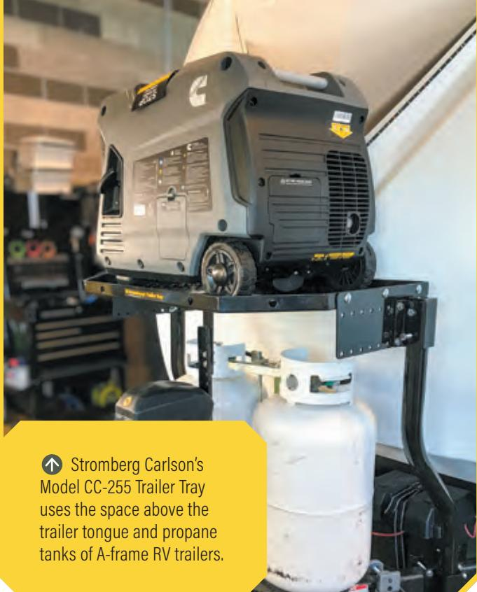
↑ Stromberg Carlson's Model CC-255 Trailer Tray uses the space above the trailer tongue and propane tanks of A-frame RV trailers.
