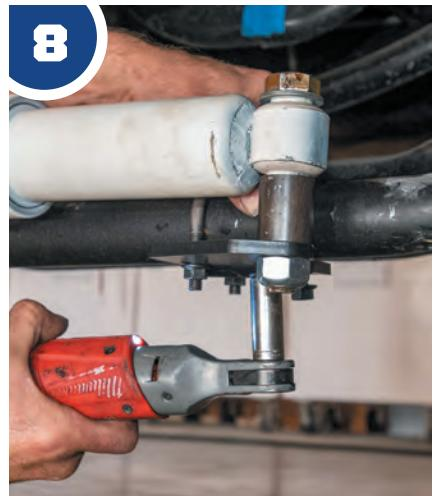
↑ The tie-rod-end U-bolt lock nuts should be torqued to 20 pound-feet after the Safe-T-Plus stabilizer is mounted to the bracket.
