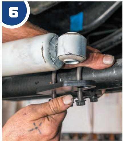
↑ The kit incorporates a special mounting bracket that attaches to the passenger-side of the tie rod using supplied  $\frac{3}{4}$ -inch U-bolts. The bracket is loosely attached with locking flange nuts.
