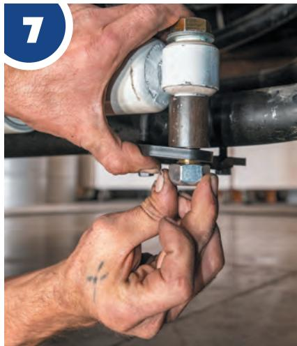
↑ The Safe-T-Plus stabilizer is secured to the tie-rod bracket using the supplied  $\frac{3}{4}$ -inch anchor bolt,  $1\frac{1}{4}$ -inch spacer, and locking nut.
